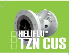
Available in stainless steel or in carbon steel. the HELIFLU™ TZN CUS flowmeters offer an accuracy better than +/- 0.15% and repeatability (+/- 0.02%), making them the clear choice for custody transfer measurement.
