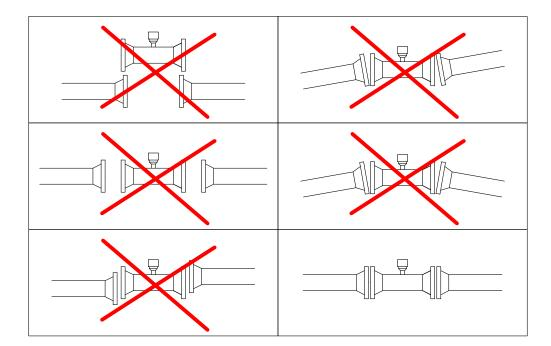
Lifting or pre-positioning means used, when necessary, shall be kept in place until installation achievement (tightening of all connecting rods).
